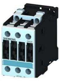
CONTACTOR, AC-3 11 KW/400 V, AC 42 V, 50/60 HZ, 3-POLE, SIZE S0, SCREW CONNECTION
